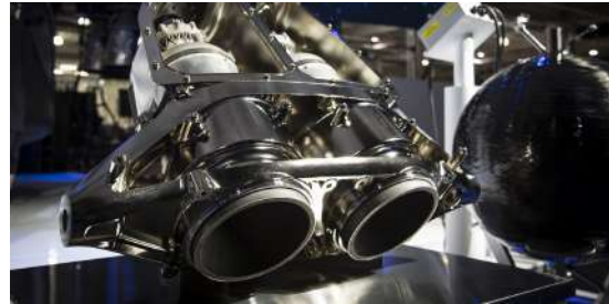
Figure H.2: SpaceX Super Draco Printed Thrust Chamber [853] (CREDIT: SpaceX)
