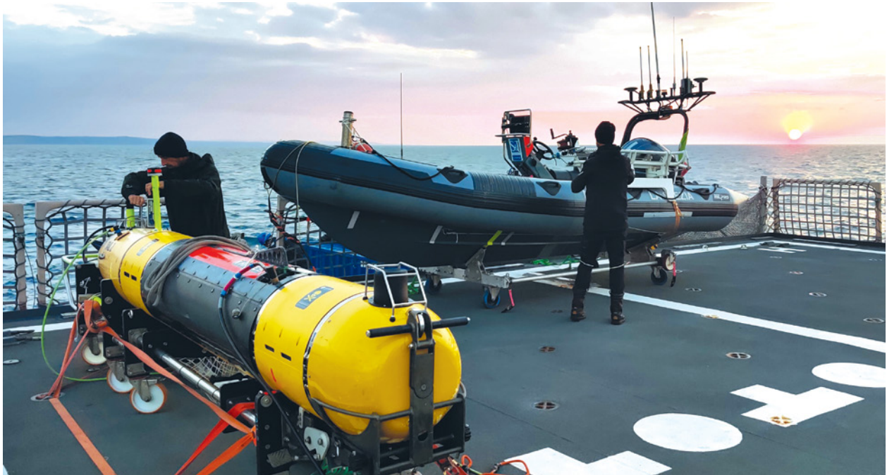
Figure 26: CMRE's MUSCLE AUV equipped with SAS onboard SPS Bam Rayo during the Naval Mine Warfare (NMW) Exercise NUSRET 21 in Turkey.
