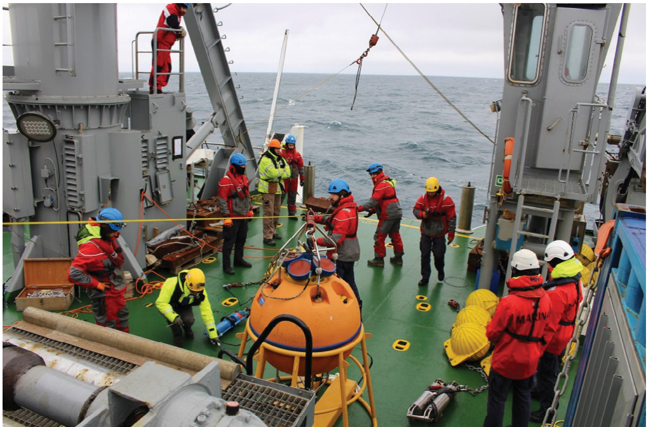
Figure 8: Deployment of a CMRE oceanographic mooring from the deck of NRV Alliance during NREP 21 campaign.
